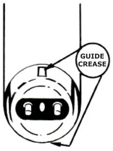
Although the lamp can be turned further into the fixture which feels like it is secure, the lamp has actually turned too far in the socket. Back off the lamp slightly until the guide creases are lined up with the opening in the lamp socket.
